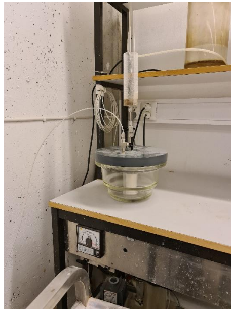
Figure 1: Core saturated with distilled water by using vacuum.
