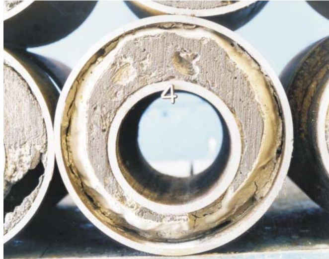
Figure: Ineffective mud displacement resulting in fluid channels. Gels in the drilling fluid have shrunk over time and provided flow paths for gas in the annulus (Watson et al., 2002).
