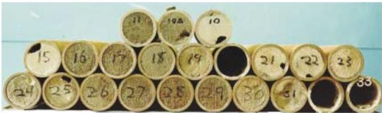
Figure 4.17: Gas channels in cement due to gas migration before cement has fully set (Watson et al., 2002)
