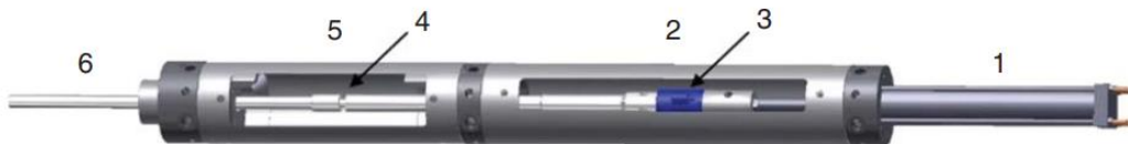
Figure 6.13: Expansion fixture system. 1 – Hydraulic cylinder with piston rod, 2 – Upper housing, 3 – Integrated-load cell, 4 – Expansion-cone spot, 5 – Lower housing, 6 – Retaining mandrel (Kupresan, Heathman & Radonjic, 2014).
