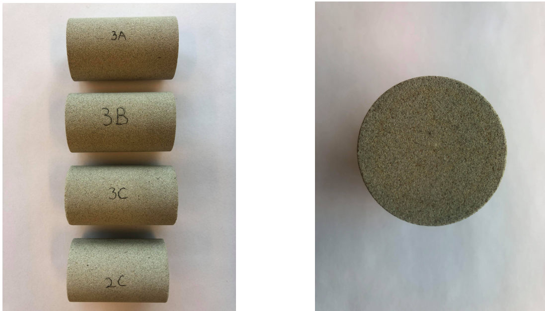
Figure 3-1: The picture to the left depicts the cores that were used in the experiments. Core 3A was used for forced imbibition with Marcol 82 as the oil, core 3B was used for forced imbibition with n-Heptane as the oil, core 3C was used for spontaneous imbibition with both n-Heptane and Marcol 82 used as the oil, and core 2C was used for spontaneous imbibition with n-Heptane as the oil. The picture to the right is of the end section of core 3A.
