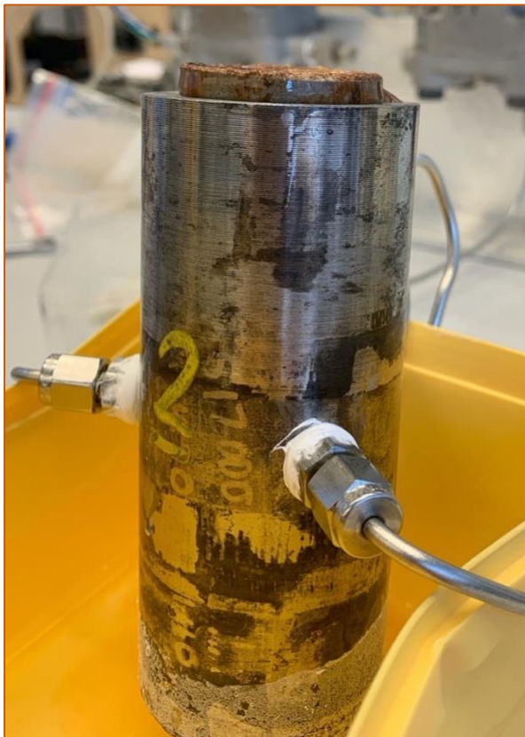
Figure 10.9 – Sample 2. Water injection through the sides. The cement core sheared at 34.47 bar. The sample is in the process of dislodging the core.
