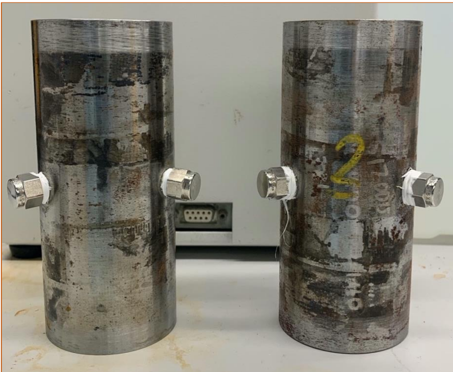
Figure 9.3 – Ports on the side of samples 2 and 3, here fitted with blinds for testing
