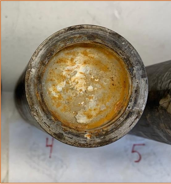
Figure 9.2 – Sample 4 after finished testing, the resin has cured into yellow/white. For illustration purposes.
