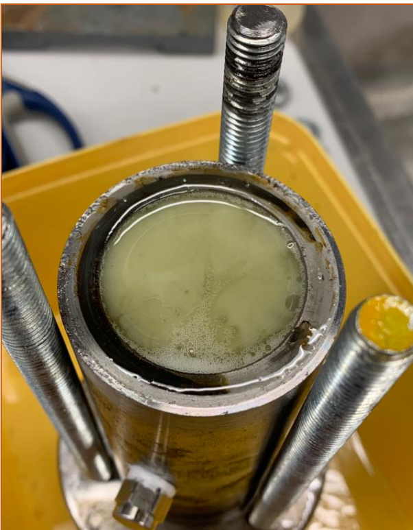
Figure 10.18 – Sample 3 disconnected after failed injection. The color of the resin is altered and there are visible bubbles in the resin.
