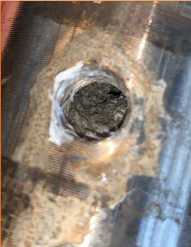
Figure 10.8 - Sample 2, the cement core appears to have collapsed from the pressure exerted by the blind plugs which was used during flow measurements.
