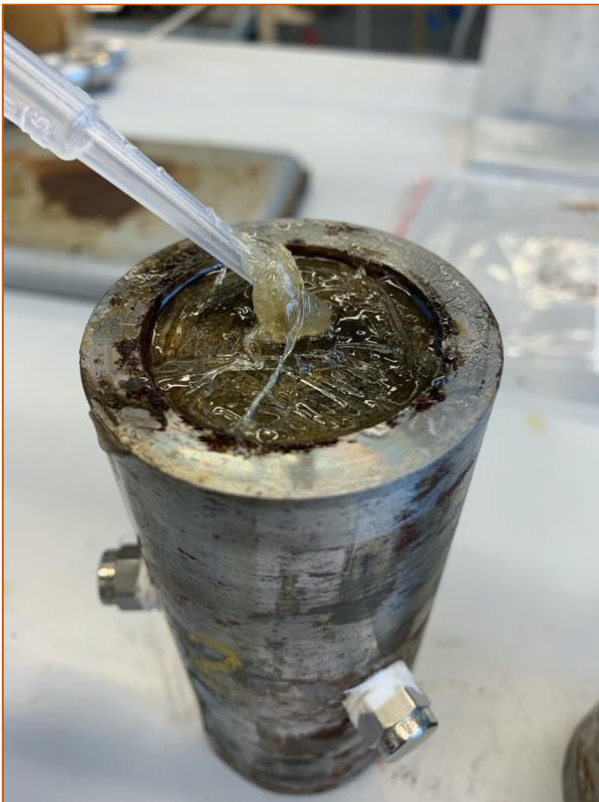
Figure 10.20 – Sample 2, residual resin is altered. It turned gel-like and highly viscous
