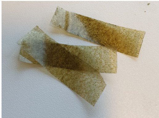
Figure 5. Alginate film with 50% seaweed cut into rectangles ready for the texture analyzer
