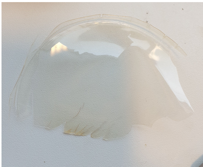
Figure 6. Example of how brittle the citric acid films treated with HPP were. The films fractured while cutting.
