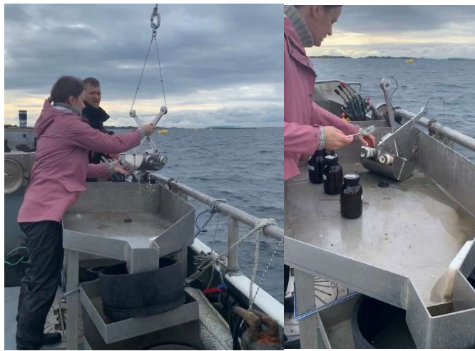
Figure 4.2-3: Van Veen Grab being used to collect sediment samples aboard the MS Scallop. (Note: This is 2020 Sampling).
