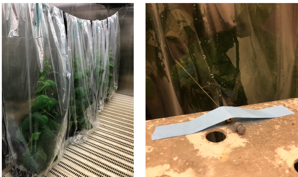
Figures 5A and B: Pictures showing the plastic tent configuration, each containing two cucumber plants, and a SPME needle piercing one of the tents with an extended fibre for the sampling of VOCs from the headspace.
