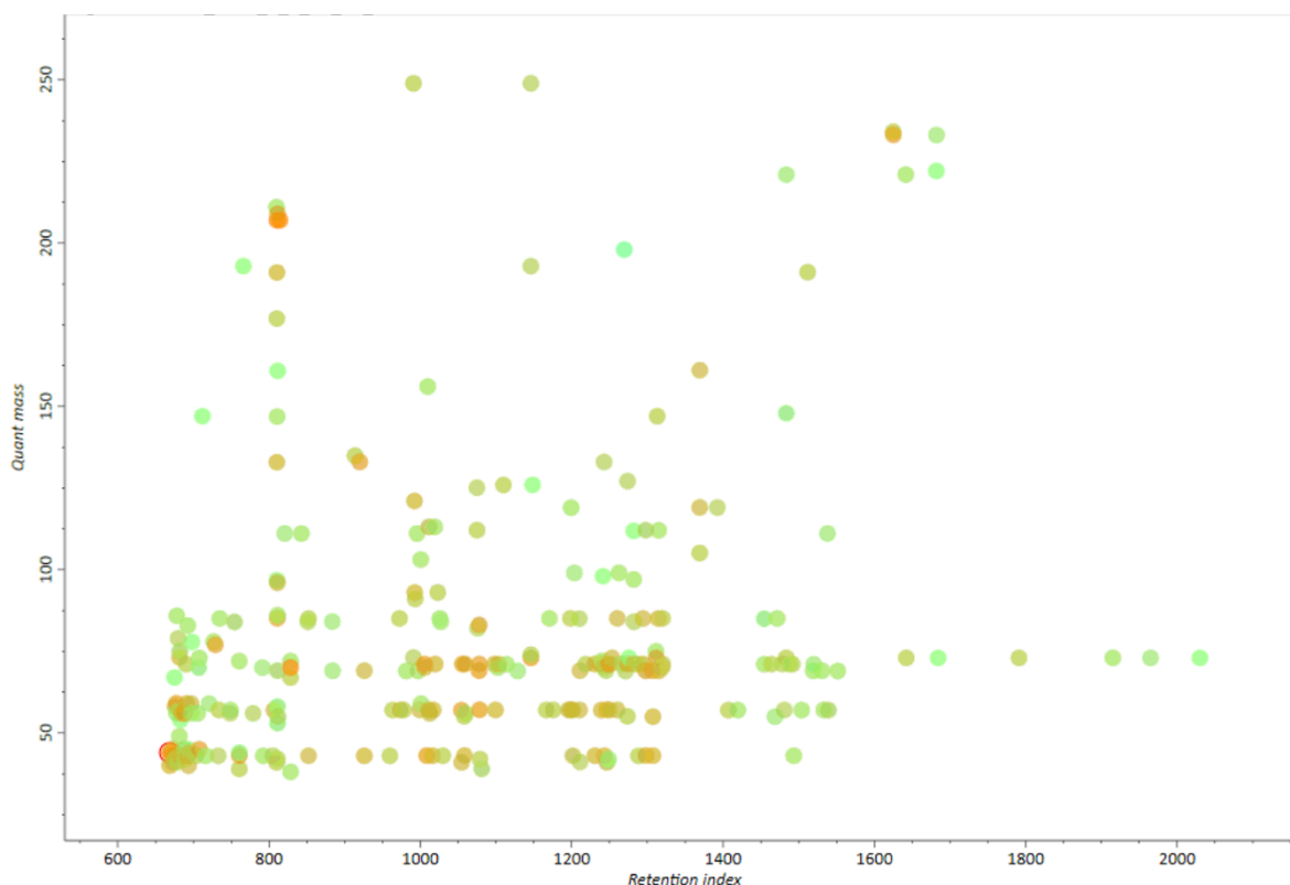
Figure 20: Alignment spot viewer from MS-DIAL before filtering and blank subtraction, displaying 259 dots which each represent an aligned peak, including retention time, quant mass and intensity. Every peak has a unique ID number, and the colours represent relative difference in peak height.
