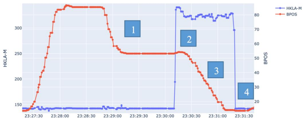
Figure 2-13. Snapshot of tripping in single stand. 1: Slip is in place during connection. 2: Drill string is connected to the hook and raised a bit to remove slip. 3: Drillstring is tripped inside the well. 4: Slip is in place for new connection.
