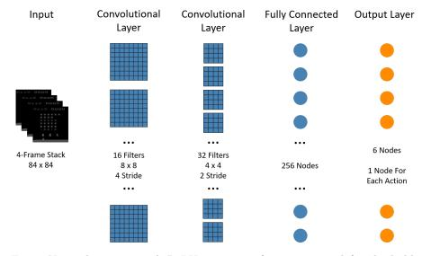
Fig. 2: Network structure. A ReLU activation function is used for the hidden layers.
