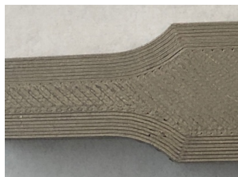
Figure 18: Raster strategy for an XY-flat subsize tensile specimen.
