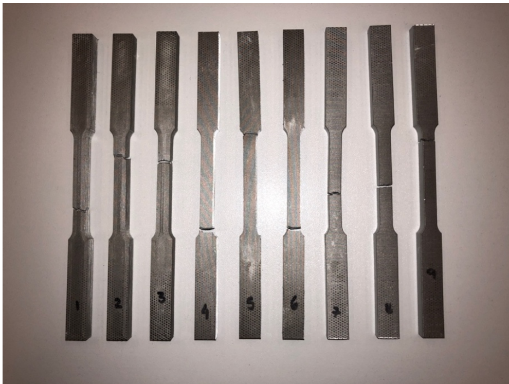
Figure 20: fracture location of all tensile specimens.
