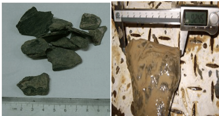
FIGURE 2.6: Any change in drilled cuttings size and shape might indicate well control problematic issues [28]
