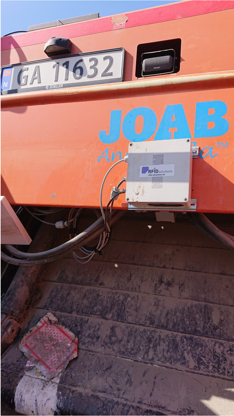
Figure 3.2: New DCU installed on truck
