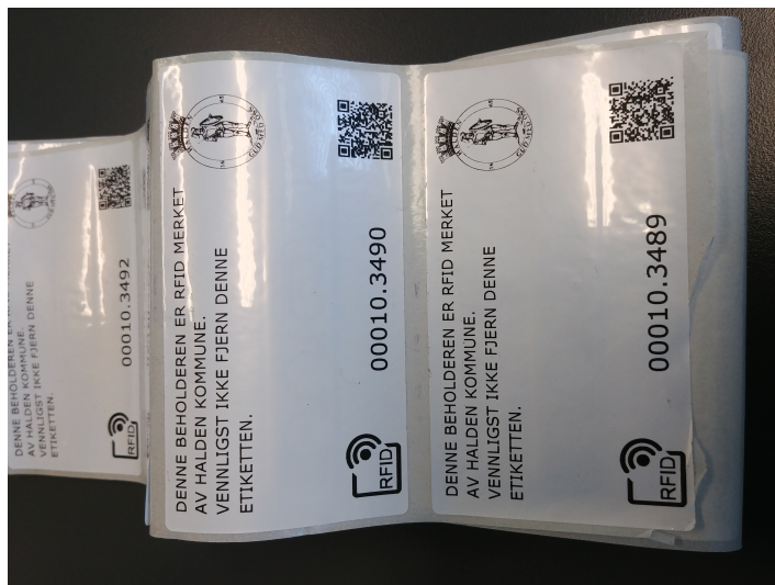
Figure 2.1: RFID Tag used by Halden on the waste containers
