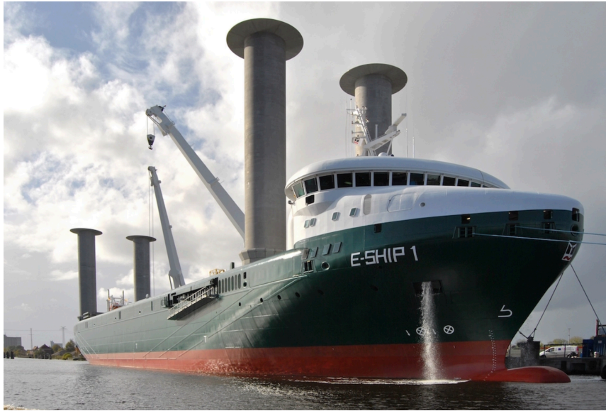
Figure 25 Flettner Rotor System installed on vessel, E-SHIP 1 [48]
