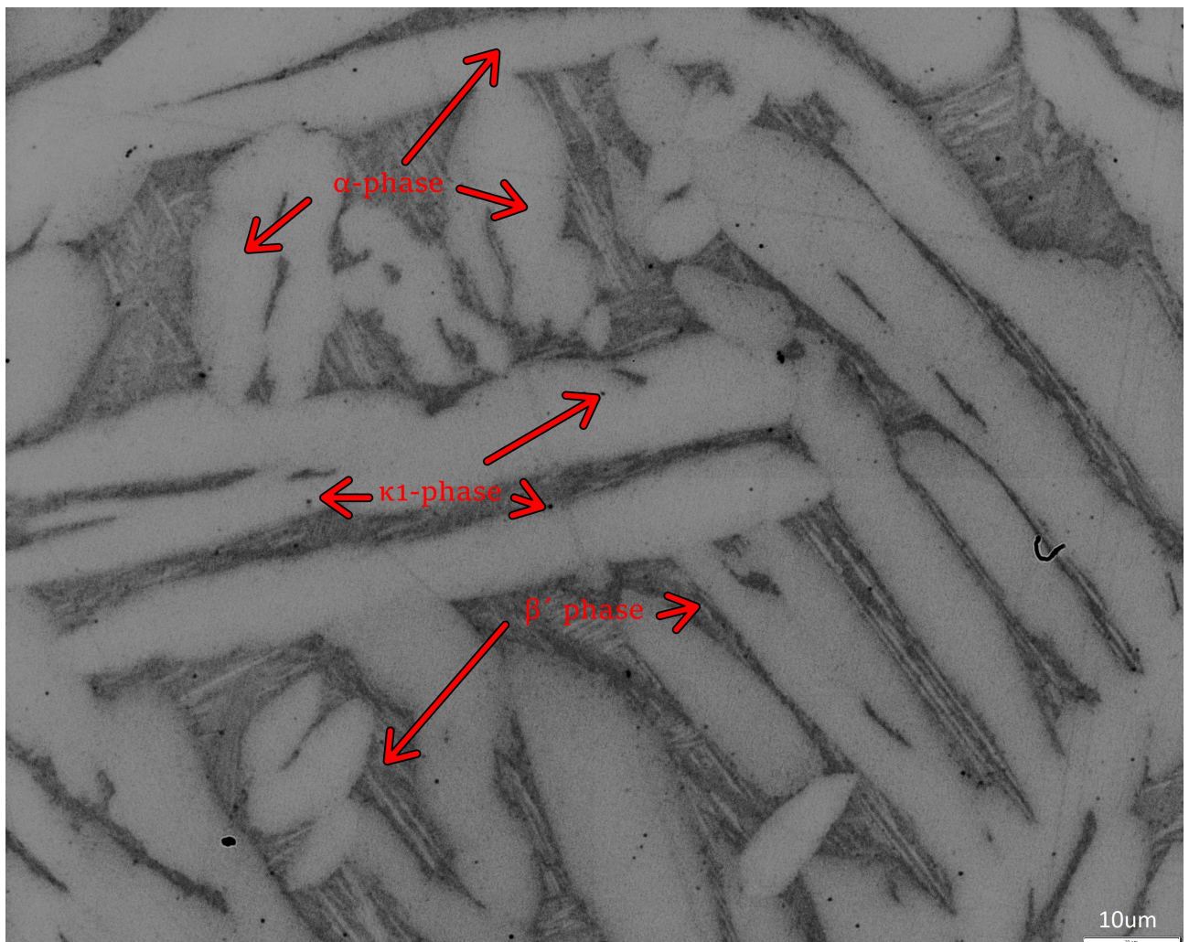
Figure 3.7.: White parts of the picture are \alpha\text{Cu} , dark lamellar are \beta' and dark dots are pores or \kappa_1 .
