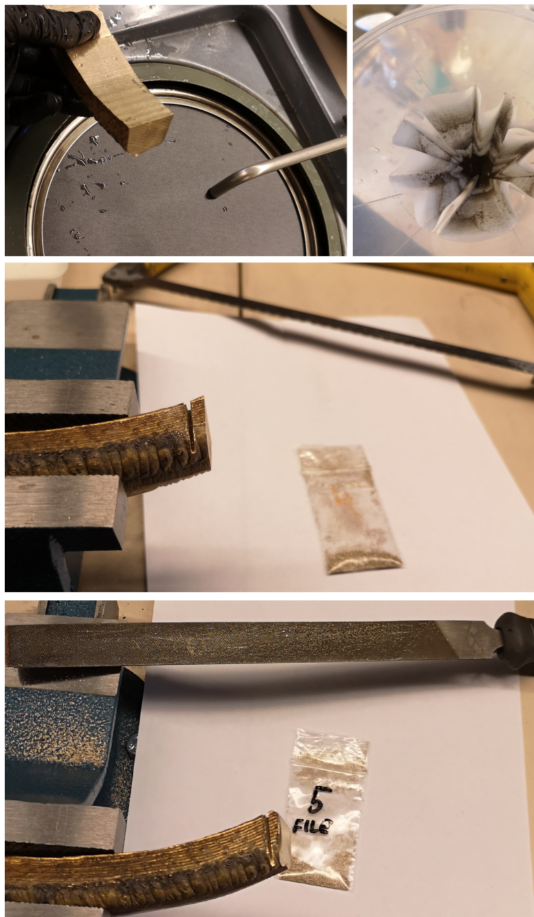
Figure 2.6.: Powder preparation for XRD - uppermost picture is grinding and then filtering of the “powder”. Middle picture is from saw cutting and the lowest picture is preparation using the file.
