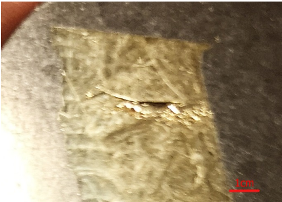
Figure 3.5.: Larger weld defect 21mm x 4mm.
