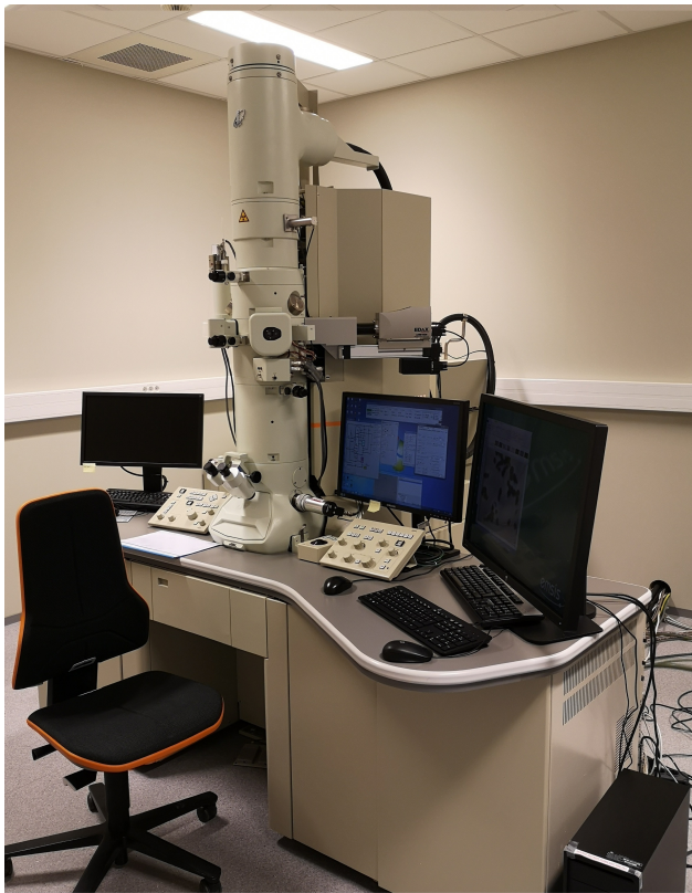
Figure 1.15.: TEM (JEM-2100) located at the University of Stavanger and the scheme of TEM [25].
