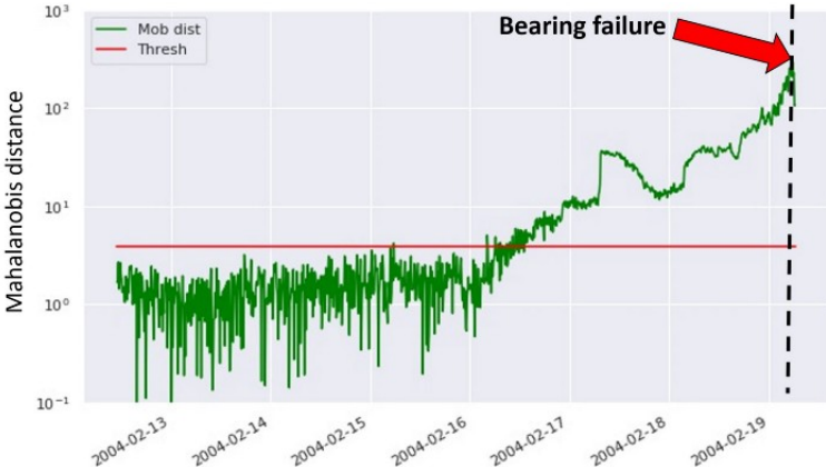
Figure 3.5: Failure of bearing over time, (Flovik 2019)
