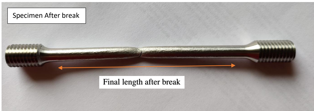
Figure 48: tensile specimen before and after the test
