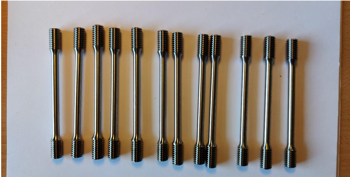
Figure 29: Prepared 316L Samples for tensile testing
