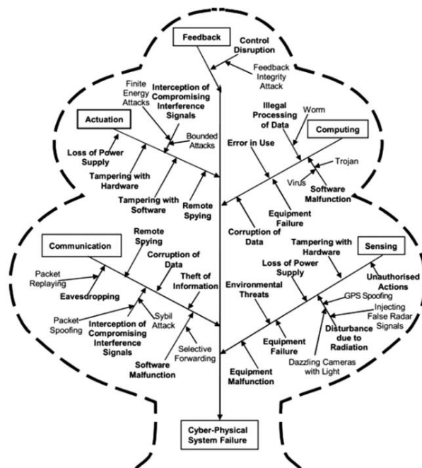
Figure 4. 4: Tree diagram of attacks and threats on Cyber Physical Systems Technologies (Maleh et al., 2019).
