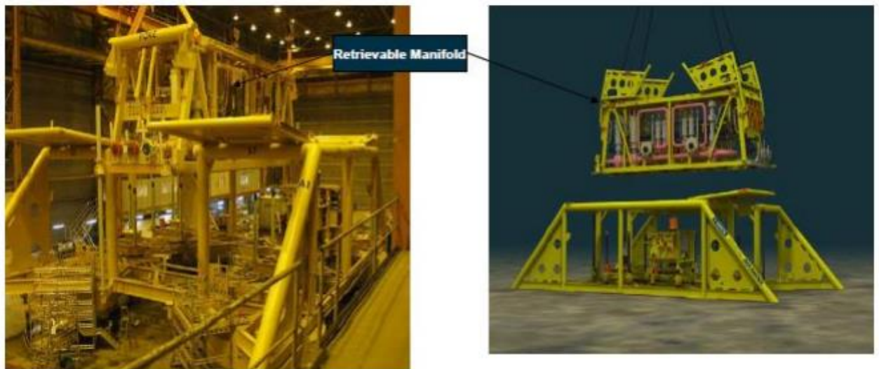
Figure 26. Manifold and template [43]
