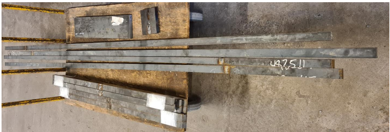
Figure 26 Test specimens after cutting
