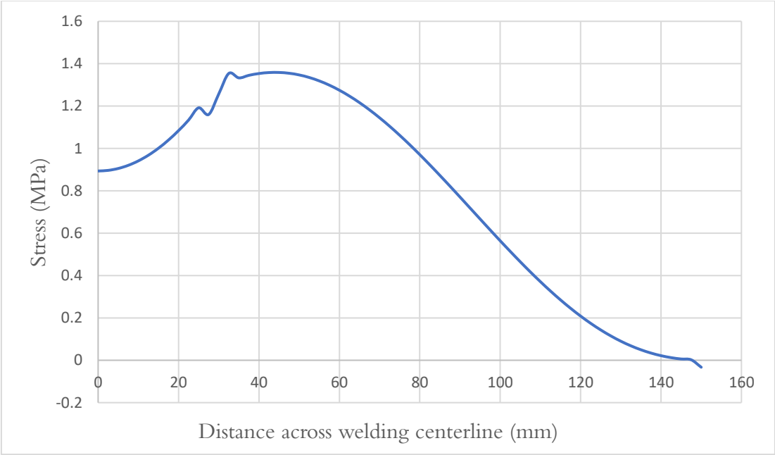
Figure 38: S11 component of residual stress across the length of the quarter plate
