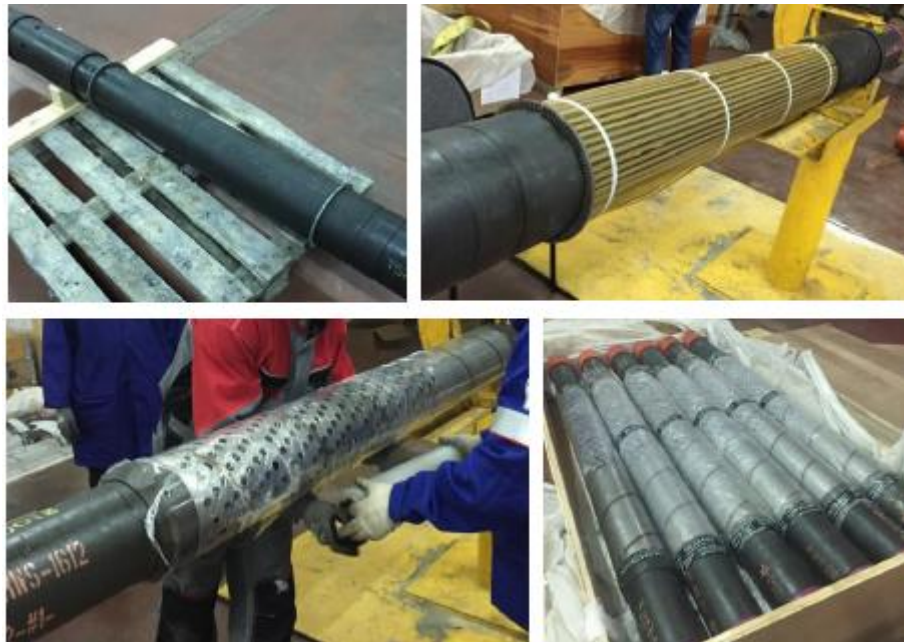
Figure 4.15 Integration of tracers into finishing equipment [8]
