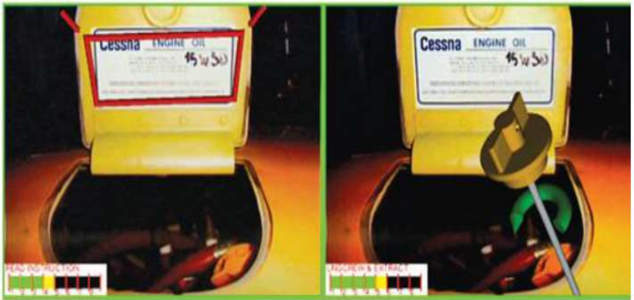
Figure 24: AR for Performing Oil Checks (De Crescenzo et al., 2011)
