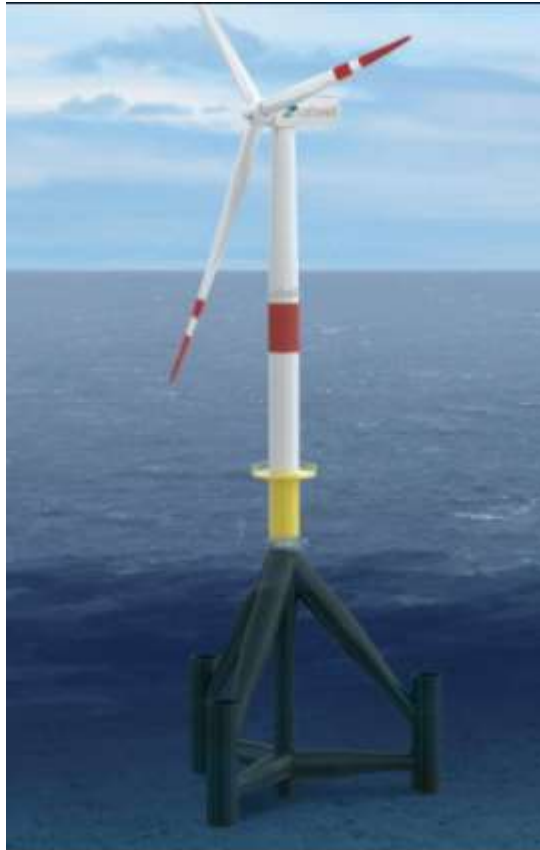
Figure 11 Tripod foundation (image by cathwell.com).
