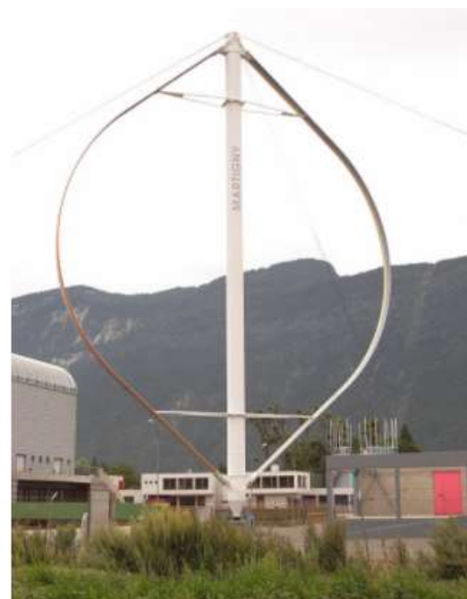
Figure 2 Darrieus vertical-axis wind turbine in Artigny, Switzerland. Source: Lysippos, Wikimedia Commons author (GNU free documentation license) (public domain)
