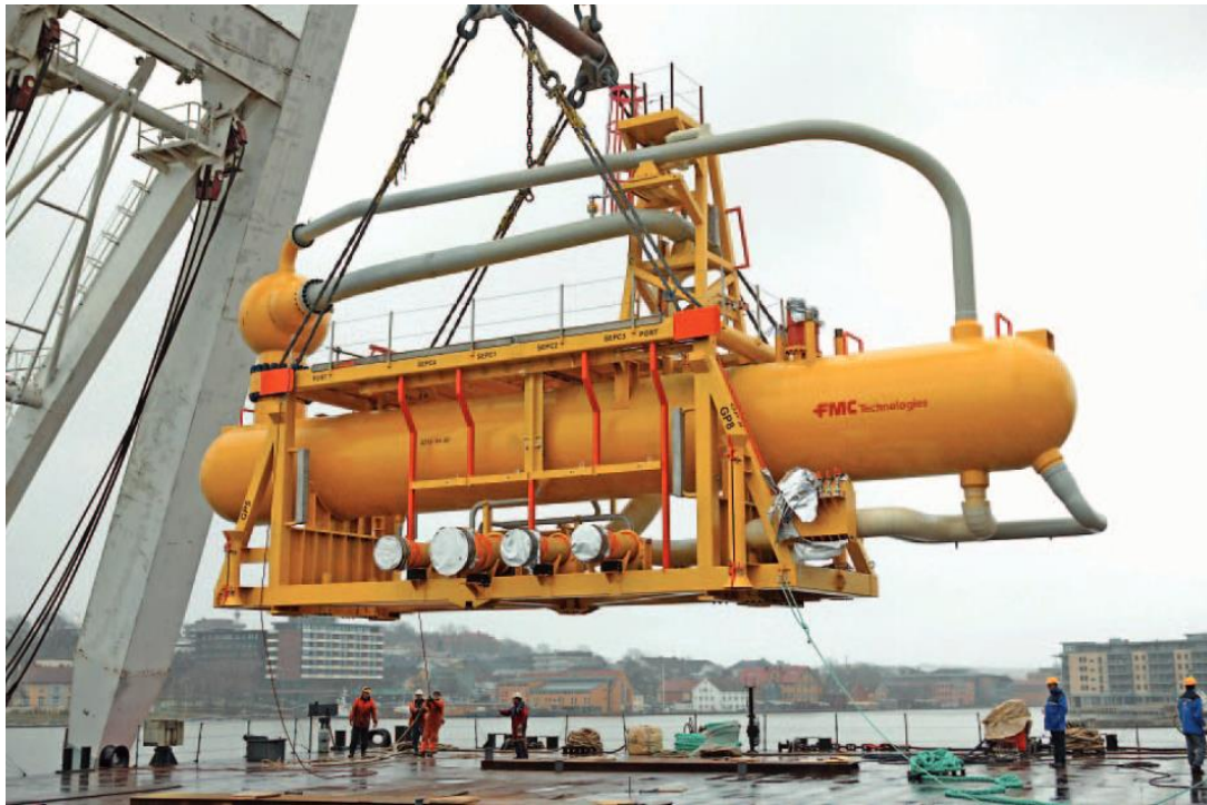
Figure 3-6 Separator for the Tordis project [12].
