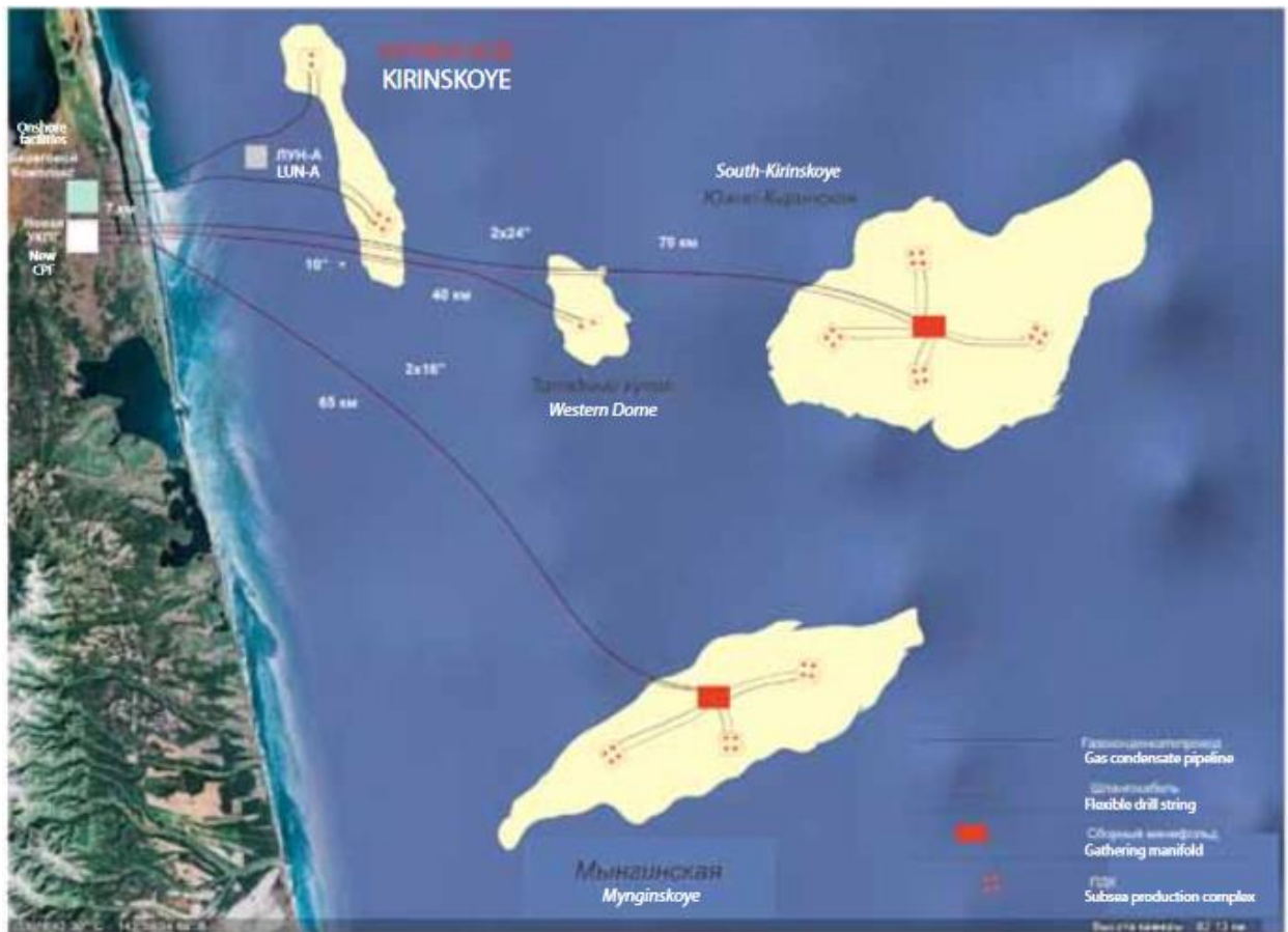
Figure 2-3 Development scheme of the Kirinskiy block including only subsea production units [7].
