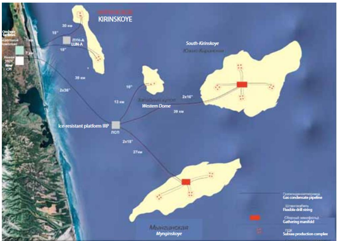
Figure 2-2 Development scheme of the Kirinskiy block including an ice resistant platform [7].
