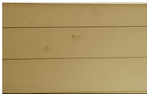
Figure 4.5: Visible dark spots on film No. 138 due to the lamp in the the Raman instrument.
