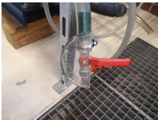
Figure E.8: Outlet valve with protractor
