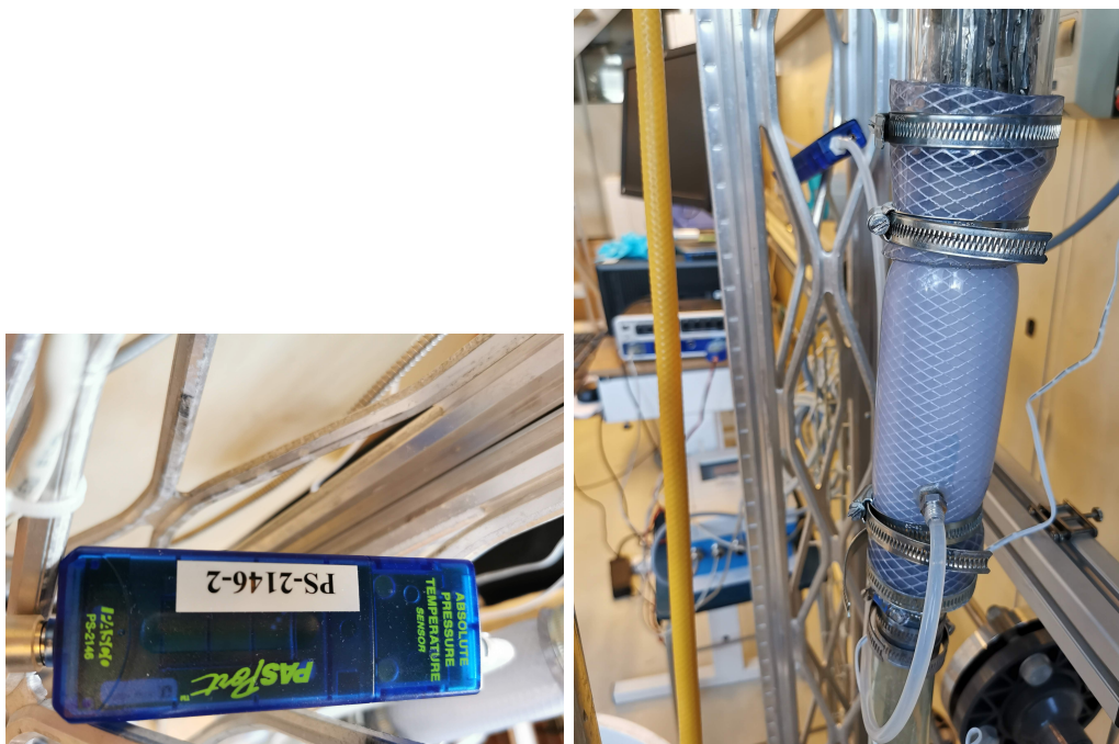
Figure E.7: PASCO absolute pressure sensor and tube coupling for the pressure sensor
