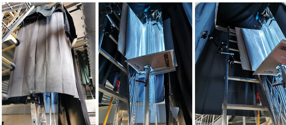
Figure E.2: Improved setup showing curtains, fish tank, and camera stand
