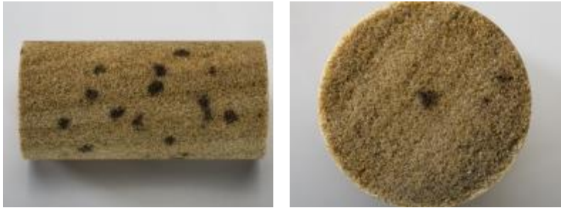
Figure 23: Longitudinal and cross sections images of a typical Leopard core sample
