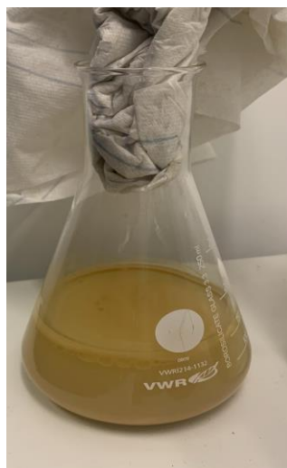
Figure 58: Effluent collected after flooding Leopard core with low salinity brine after second core restoration viscous flooding experiment
