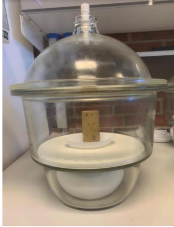
Figure 34: Leopard core sample placed in a desiccator
