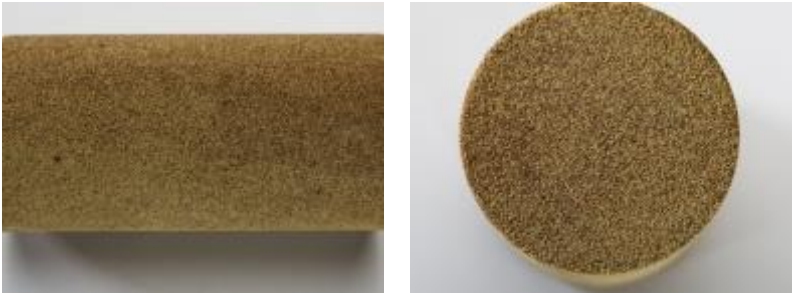
Figure 22: Longitudinal and cross sections images of a typical Bandera Brown core sample
