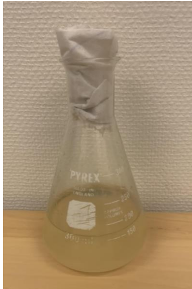
Figure 59: Effluent collected after flooding Leopard core with low salinity brine after fourth core restoration viscous flooding experiment
