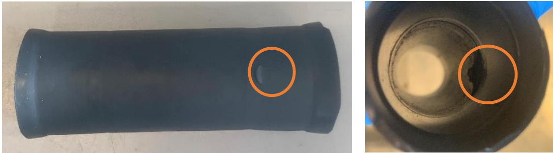
Figure 50: Longitudinal and cross sections of the punctured rubber sleeve used for BB2-4
