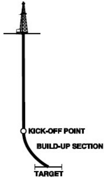
Figure 3.5: Bidimensional well trajectory of a J-shaped well. Source: (Sunny, 2015b).
