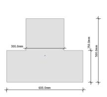
Figure 9-13 Concrete inverted T-beam (600x500)
