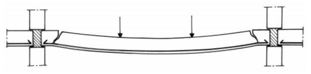
Figure 2-8 Restraining of the connection, leading to a negative moment at the support [6]
