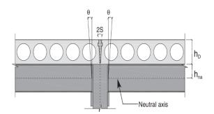
Figure 2-23 Element rotation at support [23]
