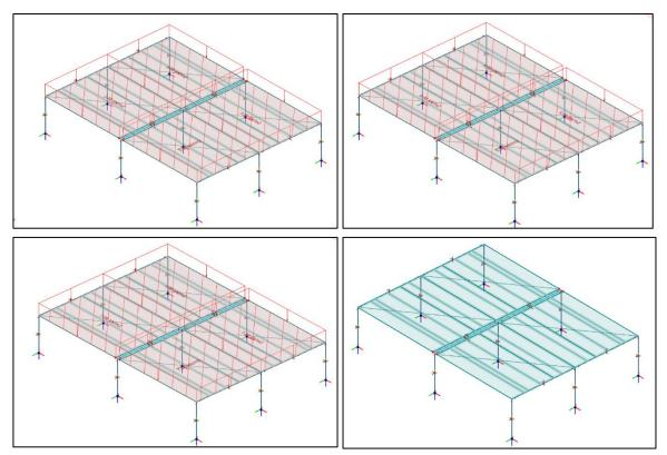
Figure 9-6 Added surface load on the HCS.
