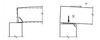
Figure 2-5 Mechanical behavior of a structural connection can be characterized by a load-displacement relationship for the primary action [6]
