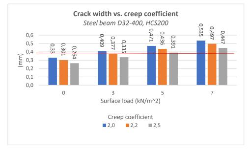
Figure 5-7 Crack width calculations with different creep coefficient
