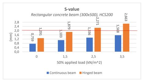
*Figure 5-10 S-value for rectangular concrete beam (300x500)*
