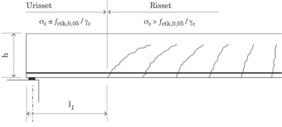
Figure 2-16 Area uncracked by bending [2]
