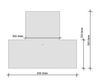
Figure 5-6 Concrete inverted T-beam (600x500)
