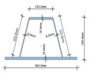
Figure 5-3 Steel beam D32-400
