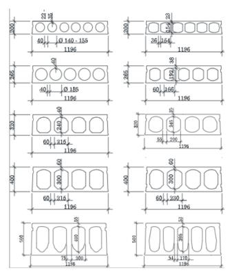
Figure 2-1 Different cross-sections of hollow core slabs [2]
