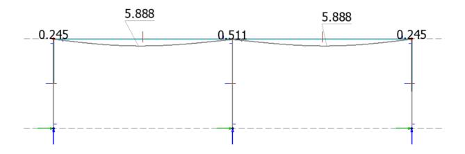
Figure 5-1 Deflection of supporting beam in FEM-design.
