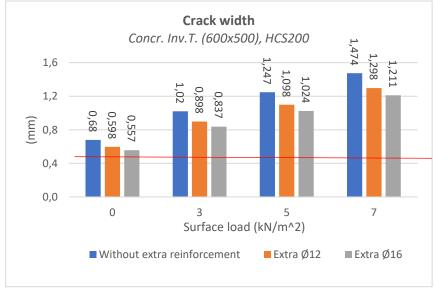
Figure 5-5 Crack width for concr.inc.T (600x500),, HCS200
