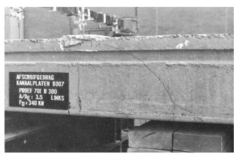
Figure 2-14 Shear compression failure [9]
