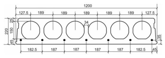
Figure 2-2 Reinforcement strands in hollow core slab [4]
