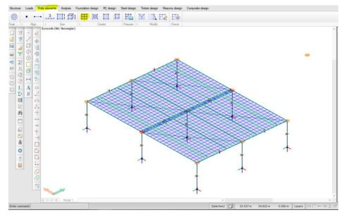
Figure 9-7 Meshing of the model
