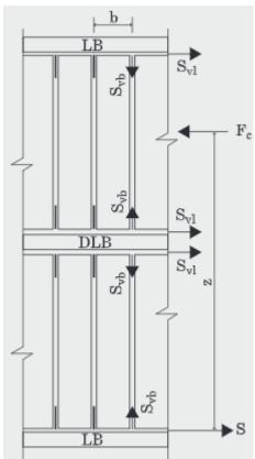
*Figure 2-11 Horizontal forces in hollow core system* [2]
