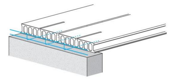
Figure 2-10 Example of reinforcement in the connection between hollow core slab and supporting beam [8].
