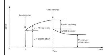
Figure 3-1 Creep in concrete
