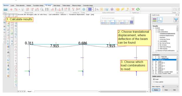
Finding the results for deflection for different load combinations are shown below.
