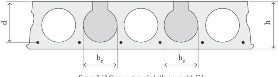
Figure 2-18 Cross-section of a hollow core slab [2].
