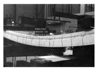
Figure 2-13 Pure flexural failure [9]
