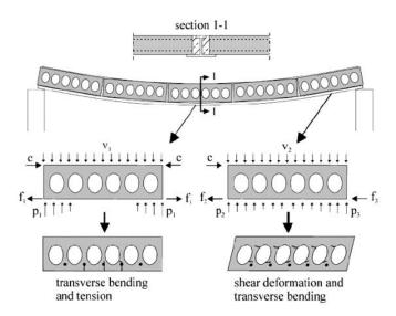
Figure 2-17 Stresses in hollow core slab on flexible support [10].
