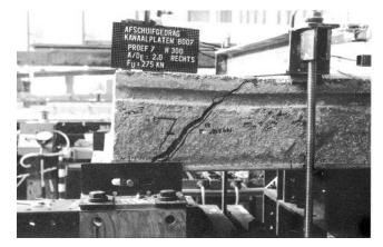
Figure 2-15 Shear tension failure [9]
