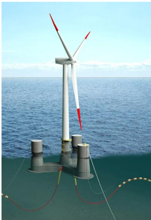
Figure 3.1 - Dr. Techn. Olav Olsens OO-Star Offshore Wind Floater[30]
