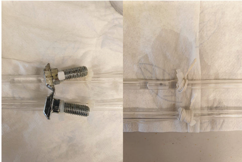
Figure C.8: Close-up temperature sensor coiled on rod and weights
