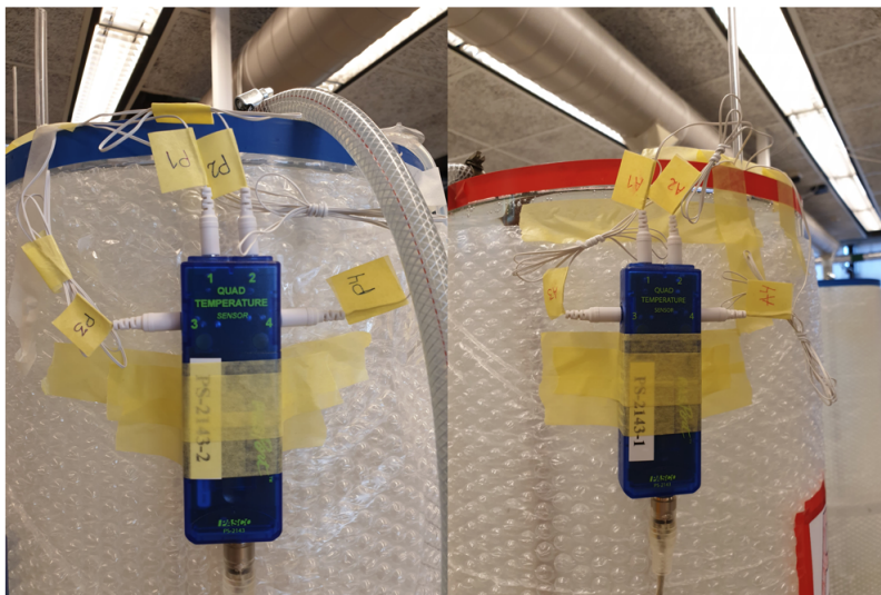
Figure C.9: Pasco Quad Sensors connected to the model
