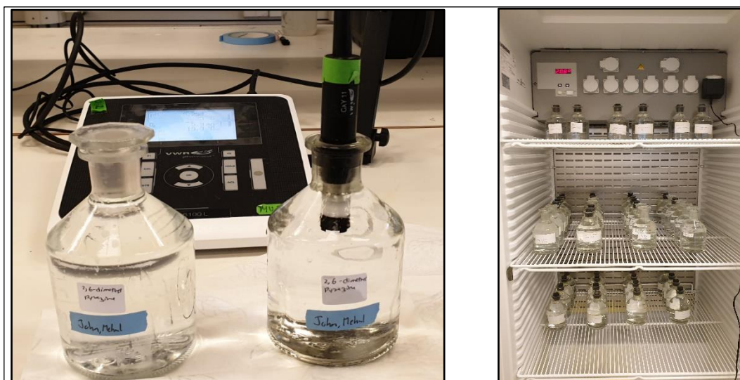
Figure 12: Measuring oxygen levels (left) and test samples stored in incubator (right).
