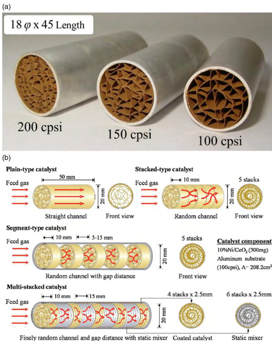
Figure 2. a) Overview of Al-honeycomb Ni-based catalysts with different cell density. Reproduced with permission. [59] Copyright 2017, Elsevier. b) Different configurations of the honeycomb catalysts: plain, stacked, segment and multi-stacked types. Reproduced with permission. [60] Copyright 2018, Elsevier.
