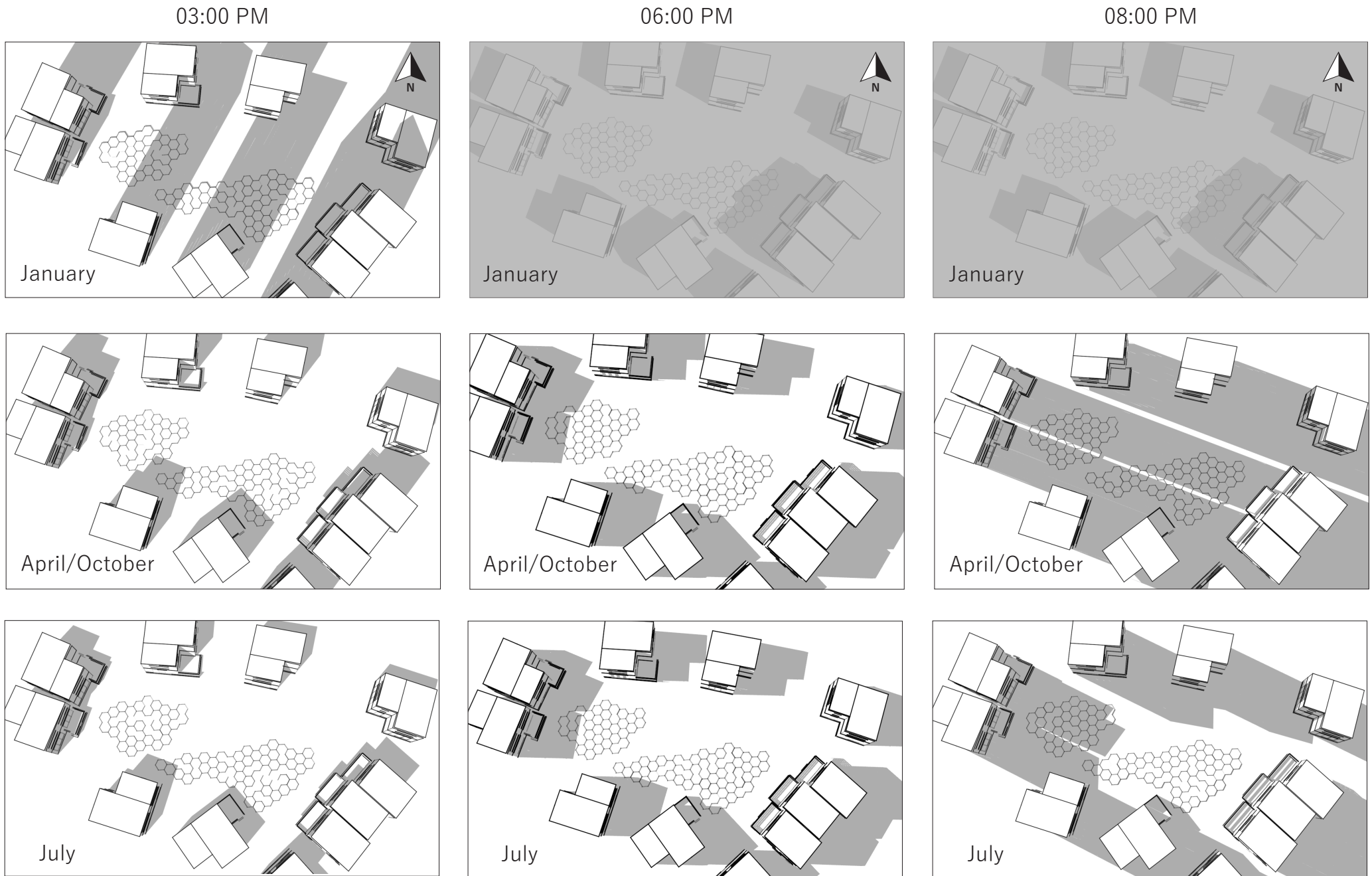
Figure 5.48: Sun conditions for the orange area at 03:00, 06:00 and 08:00 pm at every four seasons. Calculated through Sketchup with the sun and shadow tool (Self-produced).
