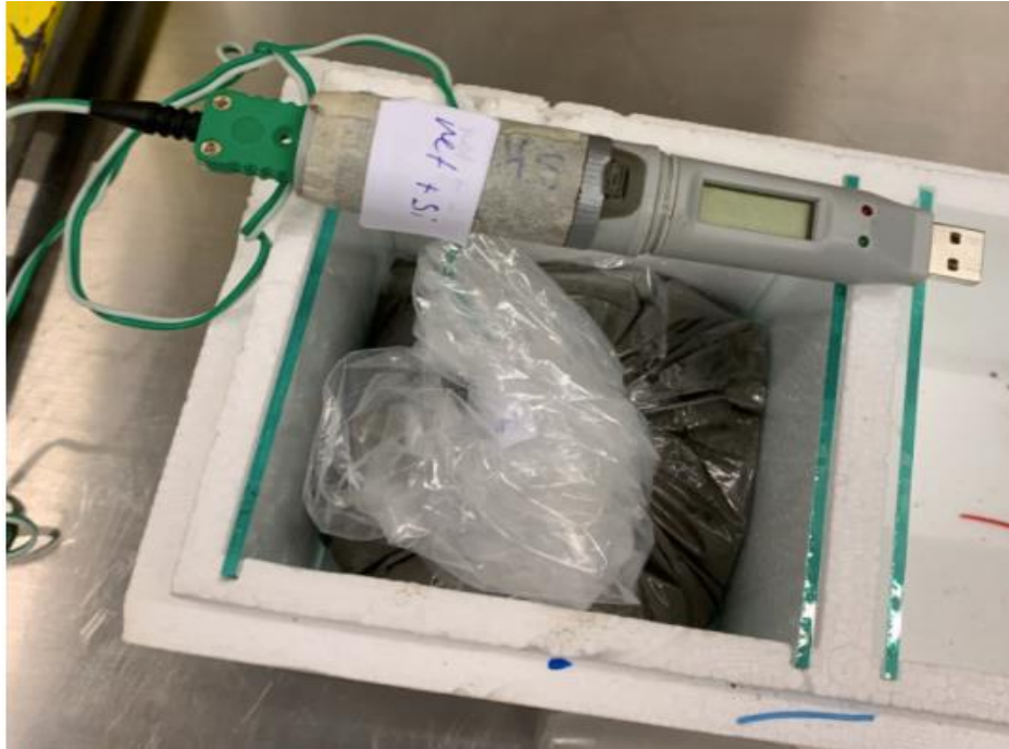
Figure 3.13 Complete set-up for measuring heat development
