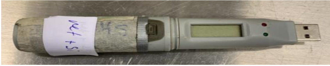
Figure 3.12 Logger used to gather temperature development
