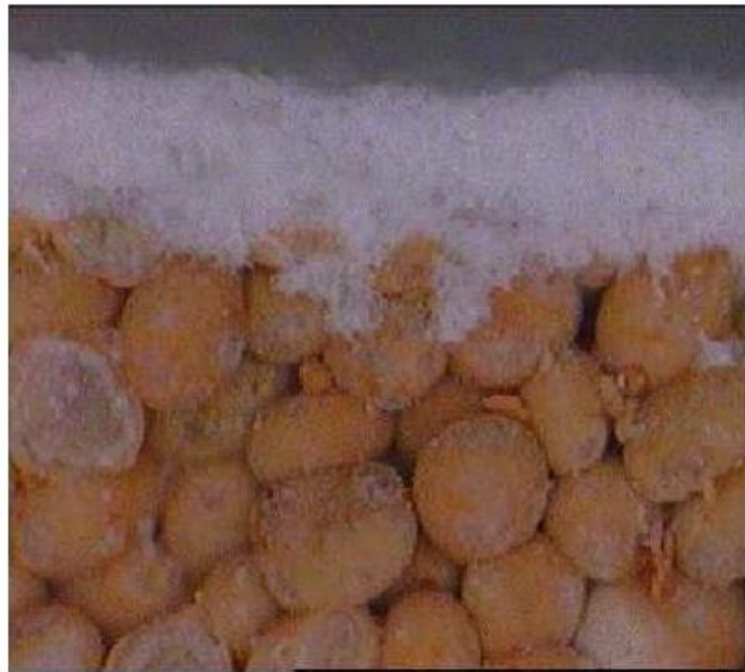
Figure 3.20: Incorrect sized \text{CaCO}_3 in drill-in fluid [49].
