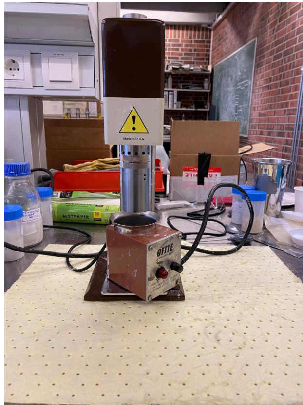
Figure 4.4: OFITE model 800 viscometer with heating cup.
