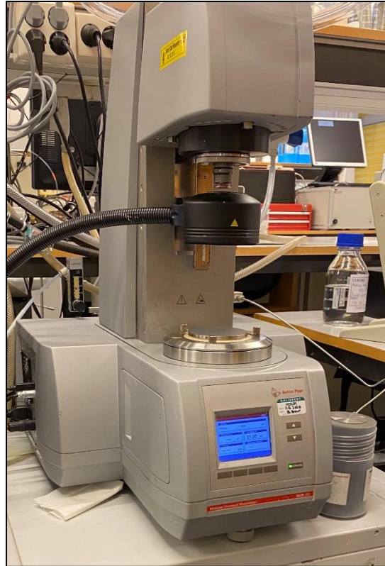
Figure 4.5: Anton Paar MCR 302 rheometer.
