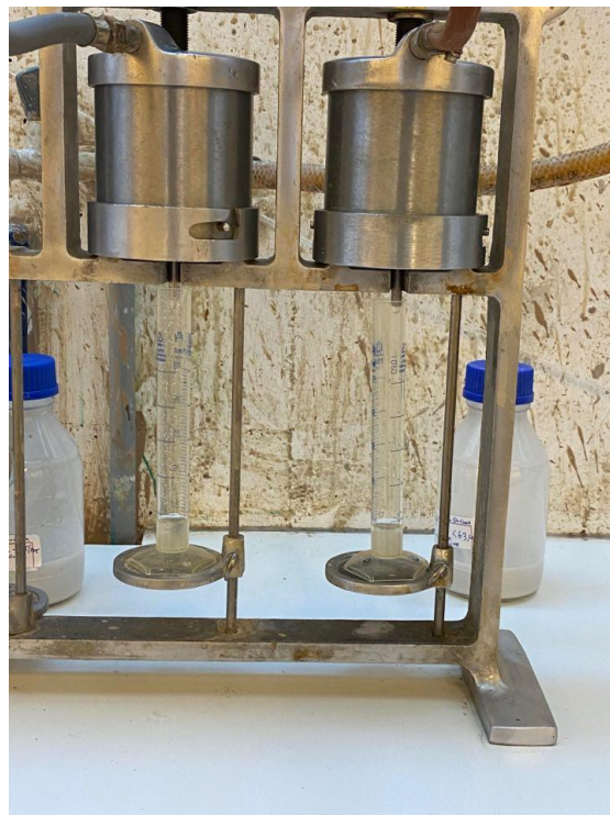
Figure 4.3: API static filter press with measuring cylinder.
