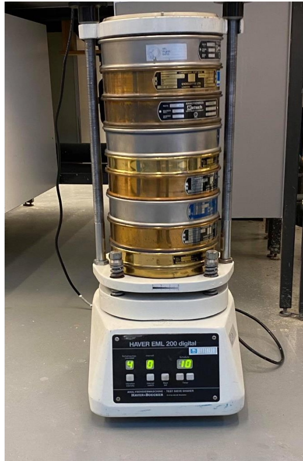
Figure 4.2: Haver EML 200 digital shaker for sieving the \text{CaCO}_3 particles.
