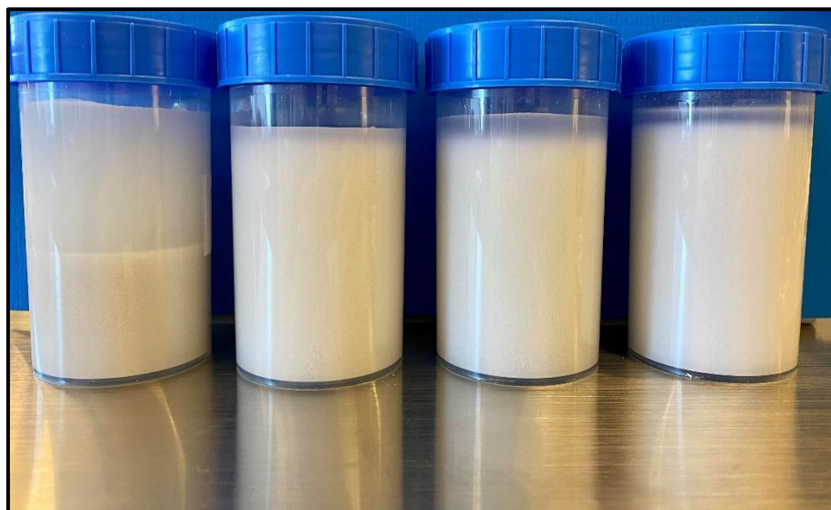
Figure 5.38: Particle stability for the cooked Na-formate reference fluid with 1wt%, 2wt% and 3wt% CaCO 3 NP's.
