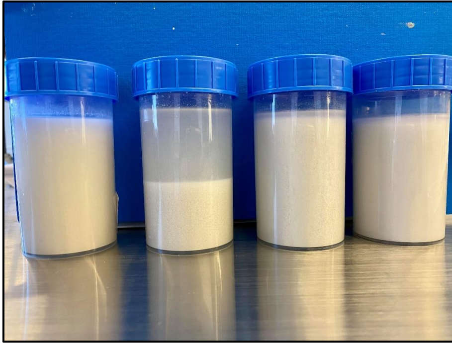
Figure 5.32: Particle stability for cooked K-formate reference fluid with 1wt%, 2.05wt% and 3wt% CaCO 3 NP's.
