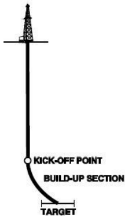
Figure 2.6: Bidimensional well trajectory of a J-shaped well. Source: (Sunny, 2015b)
