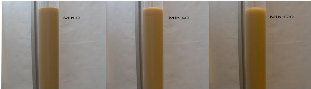
Figure 4- 7: Particle Settling schematic for 0.6 gr XG
