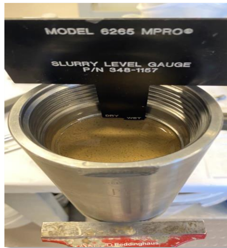
Figure 3- 14: filling level gauge
