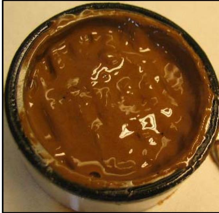
Figure 2- 1: Low-solids oil-based mud with barite left on the screen after one month (Taken from Taughøl et al., 2005).
