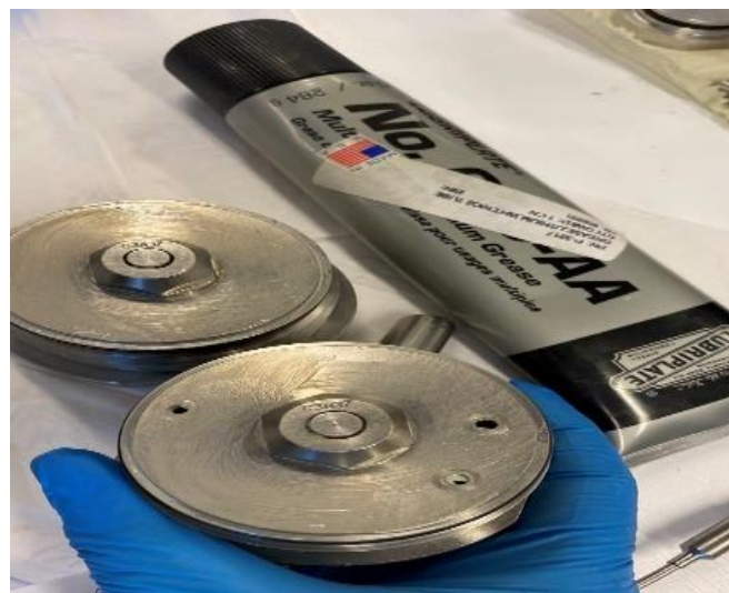
Figure 3- 13: Vessel inner surface Greasing
