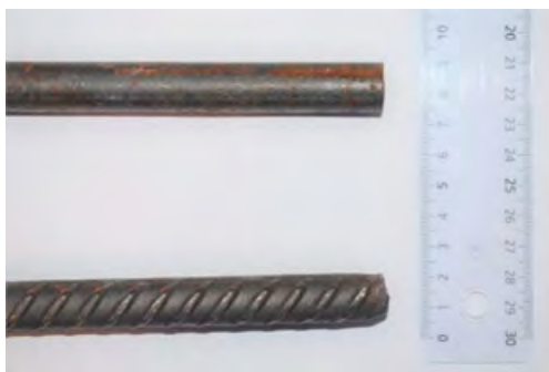
Fig. 1. Reinforcement bars surfaces of 16 mm bars used for the SS and SR.
