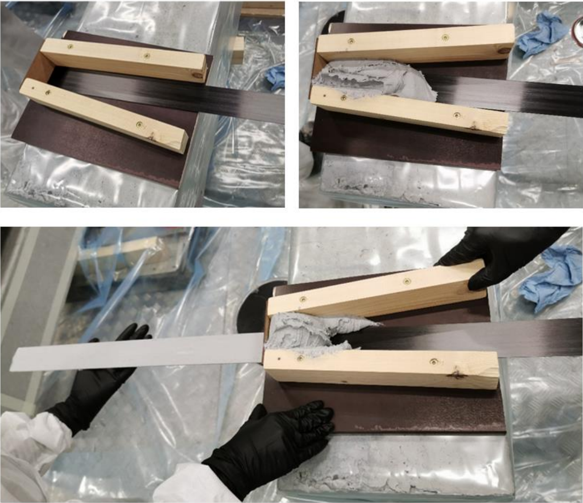
Figure 3.30 Application of the adhesive
