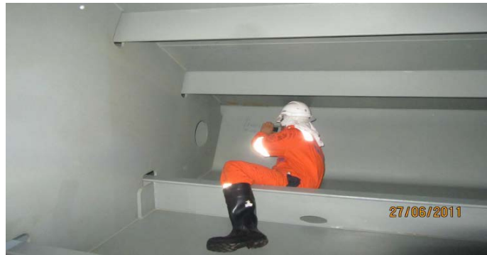
Picture 24 Ballast tank inspection by chief officer (Solvang 2012)
