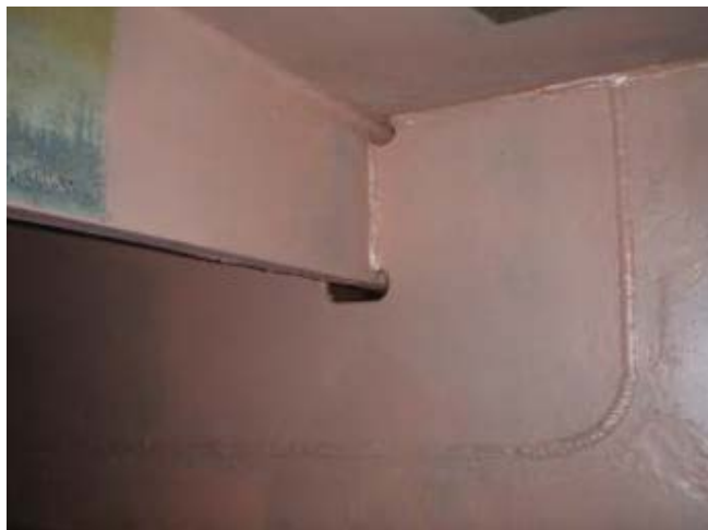
Picture 47 New insert welded in place and coated (Clipper Skagen 2009)
