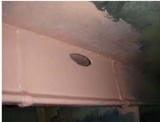
Picture 44 Renewed drain hole after coating (Clipper Skagen 2009)
