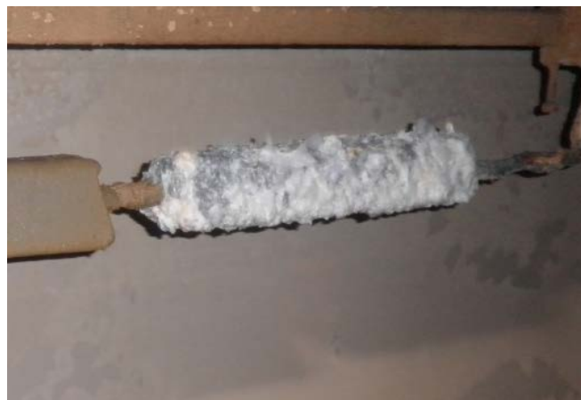
Picture 23 Zinc anode with salt deposits (Ask 2014a)
