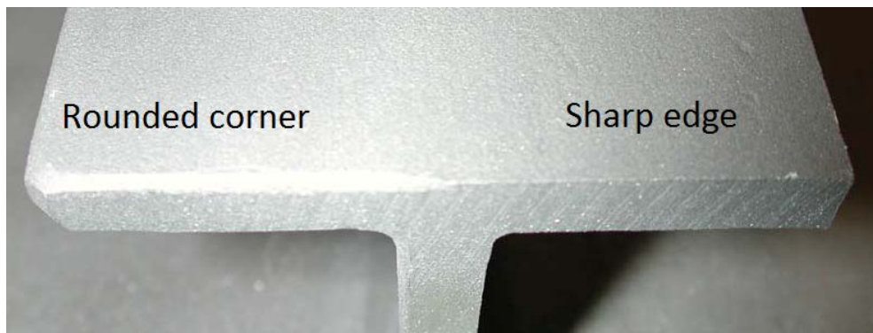
Picture 28 Rounded corner - sharp edge, painted (Solvang 2012)
