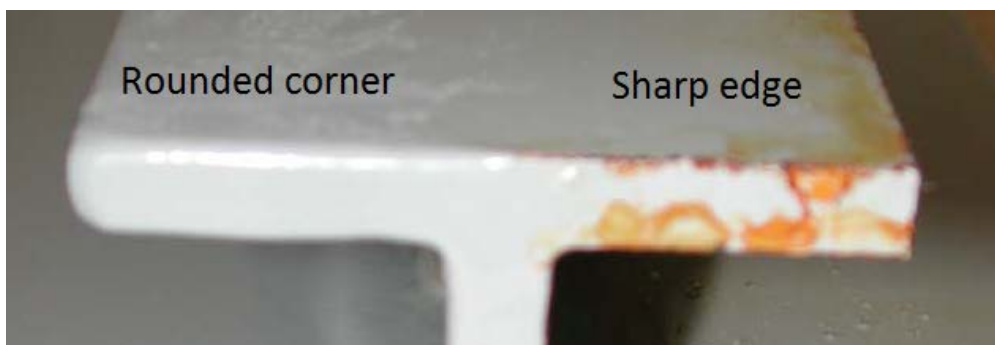
Picture 29 Rounded corner - sharp edge, 6 months later (Solvang 2012)
