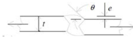
Figure 60 Butt-weld in deck-plating (DNV 2014c)
