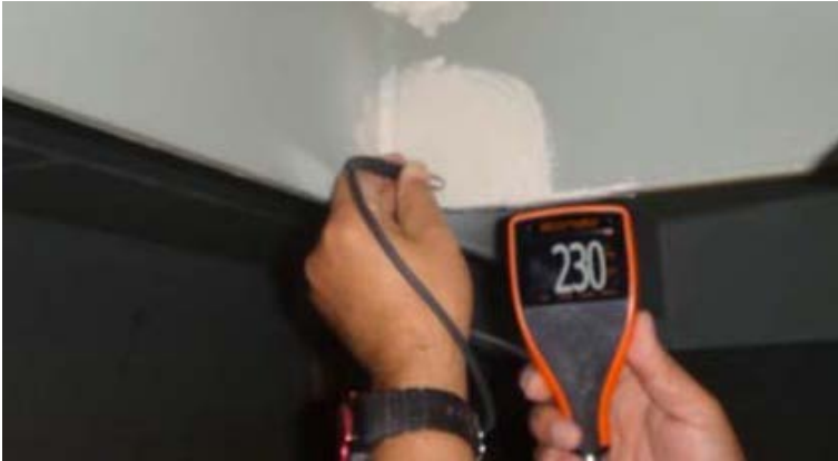
Picture 30 Thickness measurement of coating (Solvang 2012)
