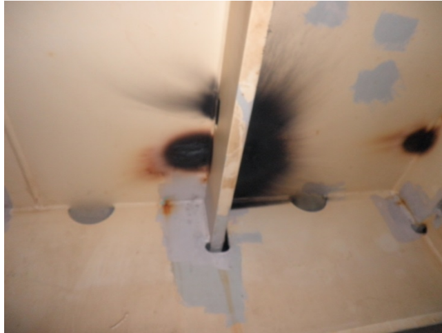
Picture 69 Deckhead after welding on deck (Ask 2014b)
