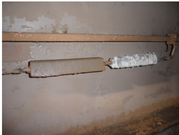
Picture 19 100% and 80% anode (Ask 2014a)
