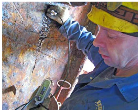
Picture 6 Technician performing thickness measurement (Cygnus 2014)
