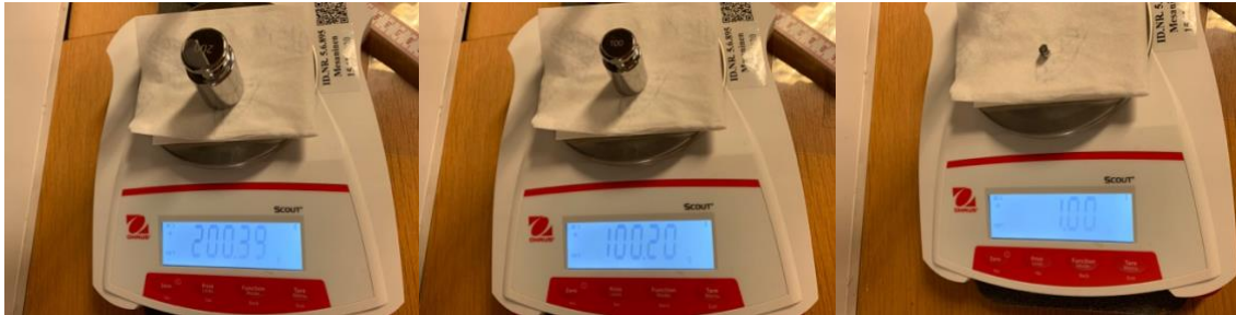
Figure 4.8: Calibration of the scale by standard weights.
