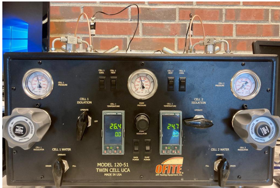
Figure 3: Model 120-51 Twin cell UCA was used for 70, 90, 110 and 130°C curing samples at 2000 psi.
