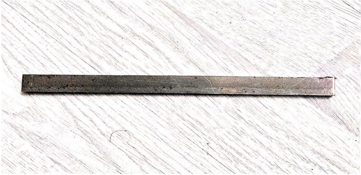
Figure 5 Sample after cutting rectangular plate using band saw machine
