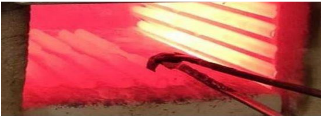
Figure 8 Samples in oven for heat treatment process
