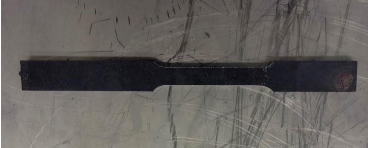
Figure 7 Specimen after CNC machining
