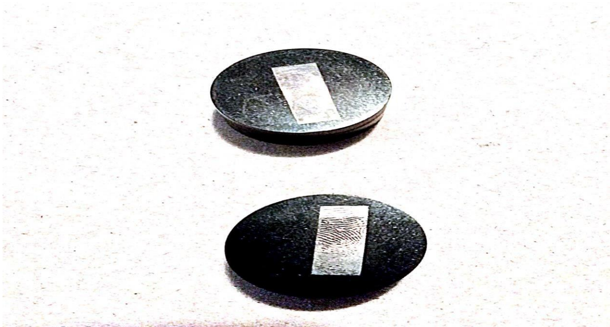
Figure 10 Plastic molded for hardness test
