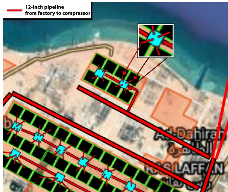
Figure 15-7: Illustration of a compressor facility(blue square) connected to 4 different ammonia plants (black squares). The red lines represent a 12-inch pipeline
