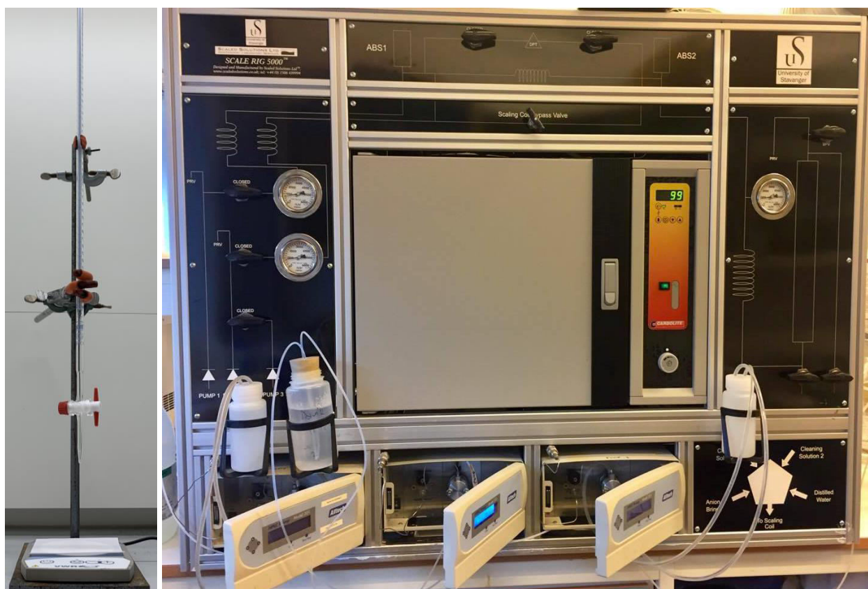
Figure 20. Titration set up for \text{Ca}^{2+} analysis by titration with EDTA (left). Dynamic scale rig used for high-pressure tube blocking testing of SIs (right).
