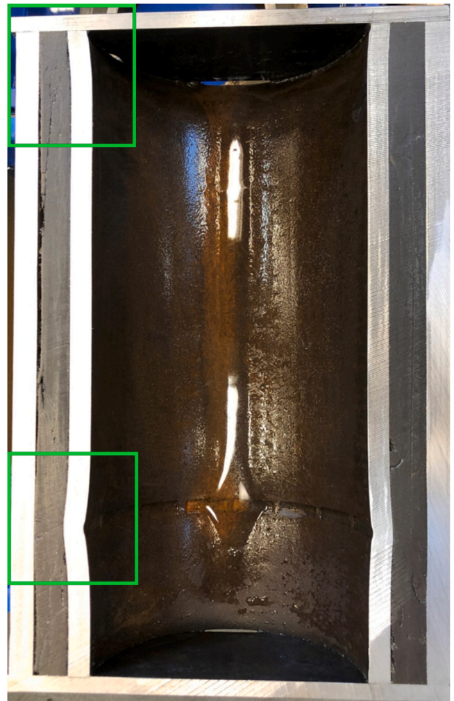
Fig. 14. Axial cross section through the dent at 1.8 m (bottom-most dent) and one half of the dent at 2.1 m (top-most dent). We observe the well-defined migration channel between the dents along the top part of the annulus (to the left in the photograph) and clear cement-casing contact areas at the levels of the two dents.
