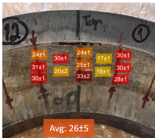
Fig. 12. Results of Vickers hardness testing in the region shown in Fig. 11.
