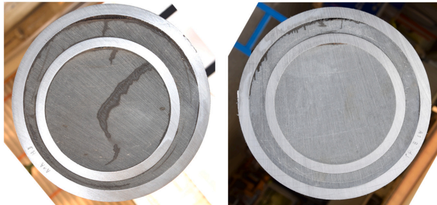
(a) In assembly A2, the eccentricity of the inner 7-in. tubing is approximately 0.45 at the left end (0.0 m) and close to centralized at the right end (8.8 m). Continuous millimeter-sized channels were present on the top side of the cement in the annulus and in the tubing.
