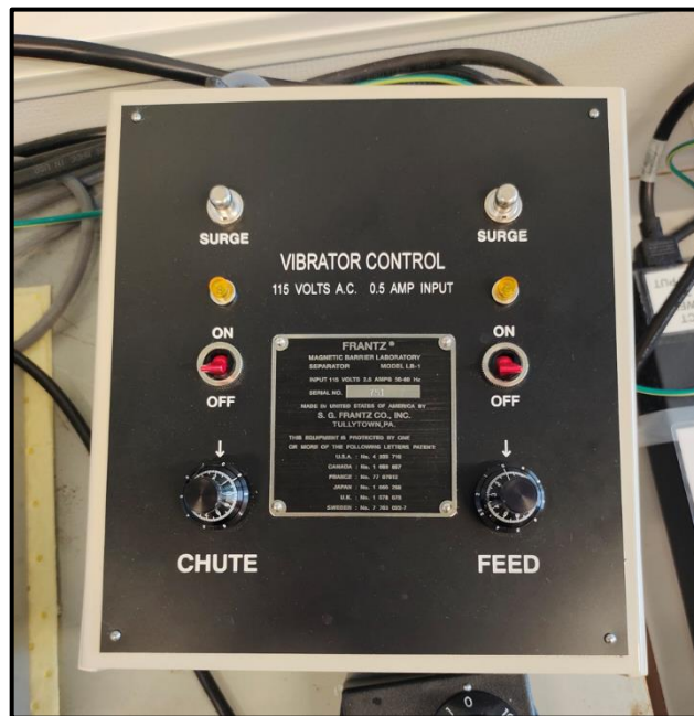
Figure 4.11 Shows the chute and feed controller to adjust the speed of feed and the vibration of the chute.
