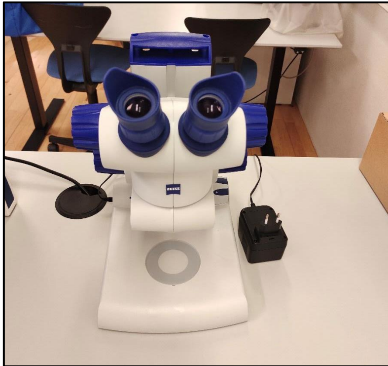
Figure 4.14 Shows a picture of a Binocular Microscope used for mounting.
