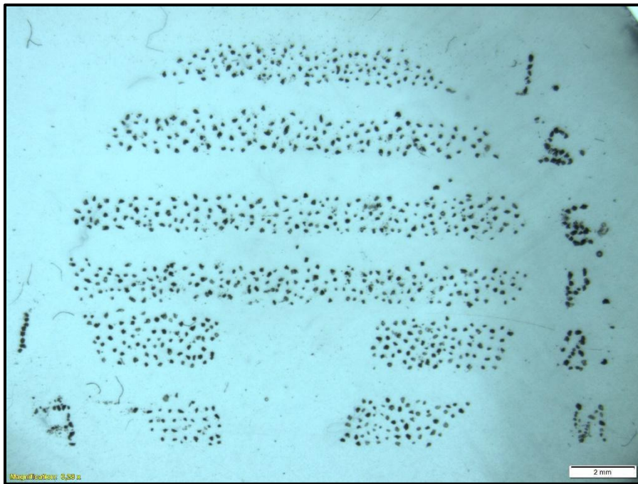
Figure 5.7 The mounted slide shows the separation of sample grains that are less than 150 microns by Frantz (R 16).
