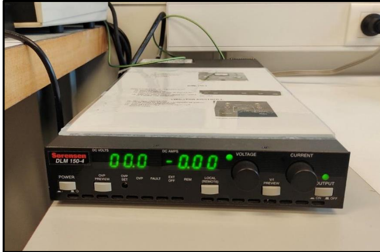
Figure 4.10 Shows the voltage controller that aids in adjusting the voltage provide to the Frantz Instrument according to requirement.
