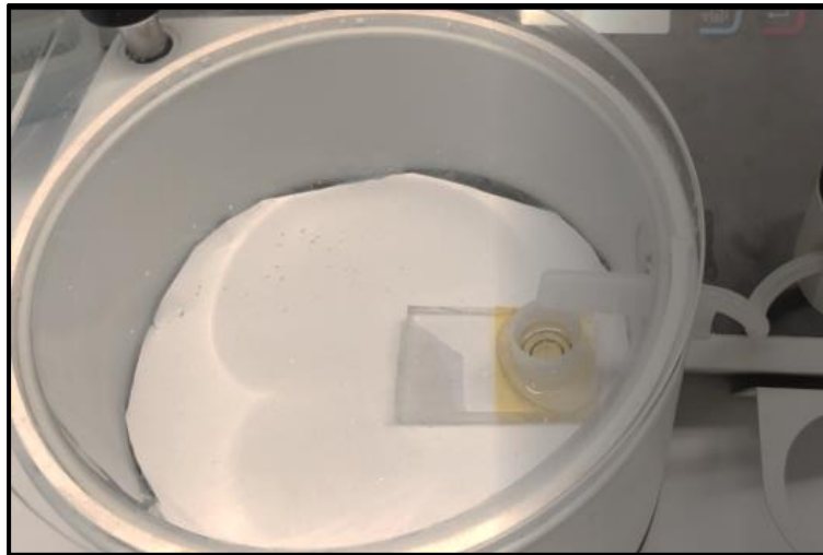
Figure 4.20 Shows the glass slide placed inside a vacuum container with a closed glass lid and epoxy flows through a pipe opening inside the vacuum.
