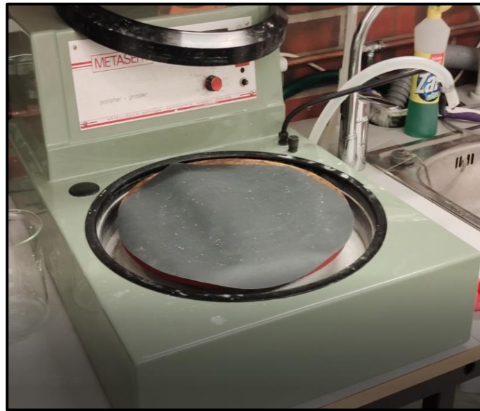
Figure 4.22 Shows the Polisher-Grinder Machine to polish the back side of the slide.
