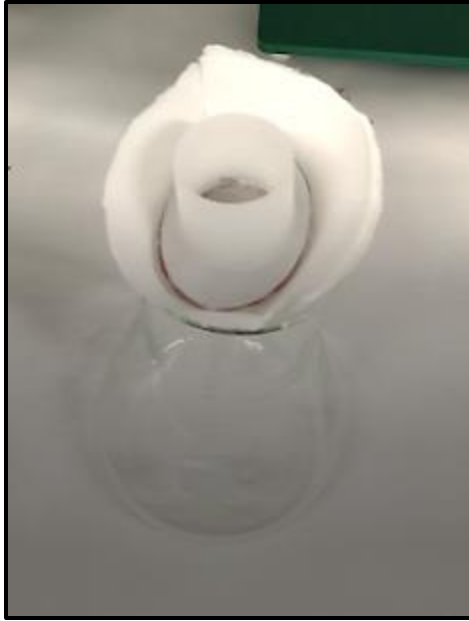
Figure 4.4 Shows the holder placed over funnel that is aligned with filter paper and placed over a flask used for sieving.
