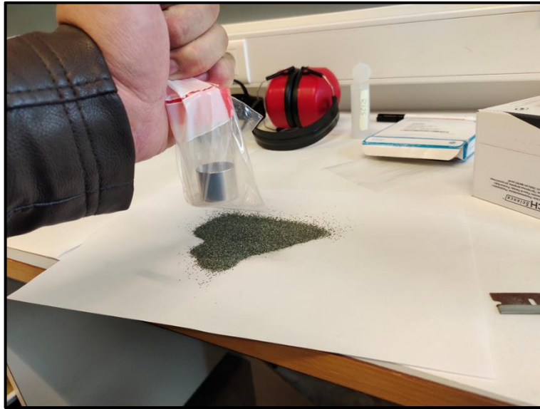
Figure 4.5 Shows the separation of ferromagnetic minerals by a magnet by hand or manually.
