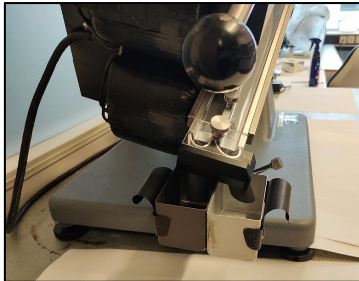
Figure 4.8 Shows two separation bins attached at the end of the chute to separate non-magnetic grains and magnetic grains.
