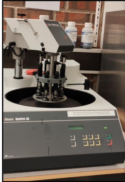
Figure 4.23 Shows Struers Rotopol-35 instrument used specifically for polishing and grinding.
