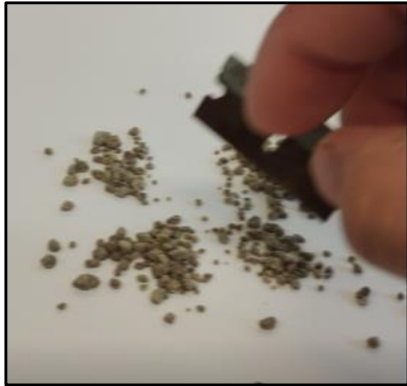
Figure 4.1 Shows the distribution of section of a sample in four different mounds of equal proportions with the help of a blade.
