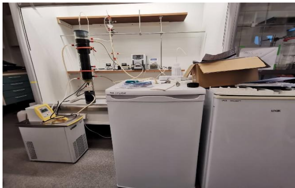
Figure 3.2 a wider photo of the UASB apparatus.
