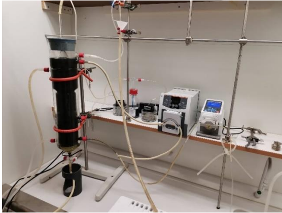
Figure 3.1 Photo of the laboratory scale UASB Reactor
