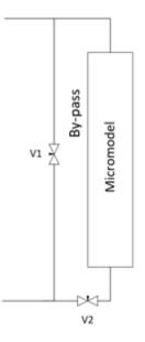
Figure 6. Valve system connected to the micromodel.
