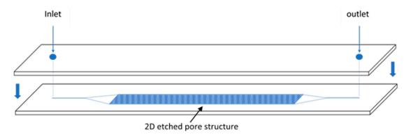
Figure 3. Sketch of the two-dimensional (2D) etched pore structure glass plate and flat glass plate design.
