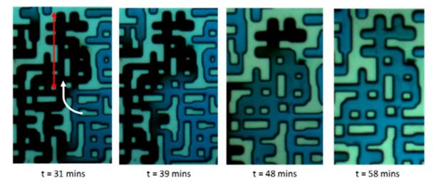
**Figure 11.**  $CO_2$  mixing upward into dead-end pores located at 14.5 mm from the top of the micromodel in Case 1. Location identified by the red circle in Figure 9 at t = 31 min.
