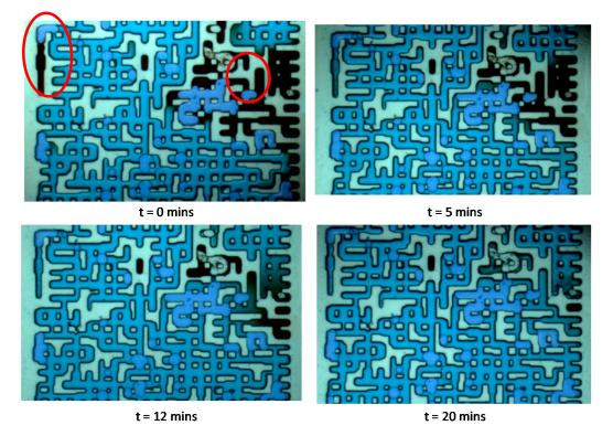
**Figure 14.** CO<sub>2</sub> invading dead-end pores through oil ganglia in the water phase (focused points in red circle), in Case 2 experiment. Location at 19–24 cm from the top.
