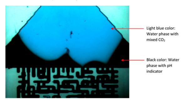
Figure 7. CO<sub>2</sub> in the triangle area when CO<sub>2</sub> injection into the micromodel was stopped.
