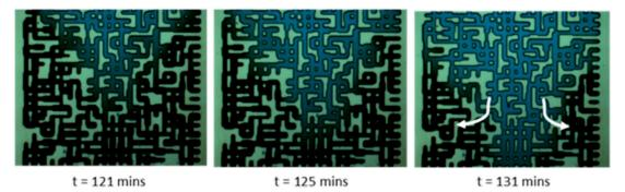
**Figure 10.** CO<sub>2</sub> transport inside the micromodel at a location 33–40 mm from the top of the micromodel, in Case 1.
