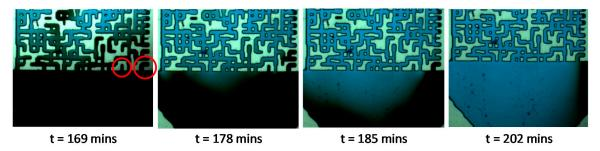
Figure 12. CO<sub>2</sub> breakthrough at the bottom of the micromodel, in Case 1.
