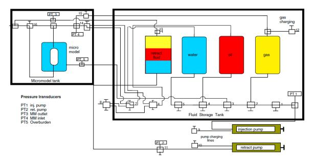
Figure 2. Schematic piping and instrumentation (P&ID) diagram of the experimental setup [31].
