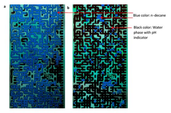
Figure 13. Micromodel image at location 10–25 mm at (a) S<sub>wi</sub>; (b) S<sub>or</sub>, in Case 2.
