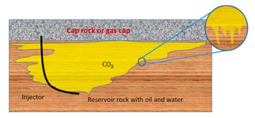
Figure 1. Simplified sketch of convection-driving dissolution of CO<sub>2</sub> with oil inside the reservoir.
