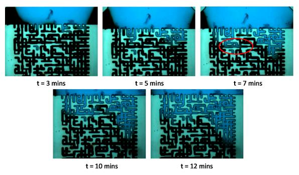
**Figure 8.** Initiation of  $CO_2$  mixing from the top of the micromodel and propagation downwards, in Case 1.
