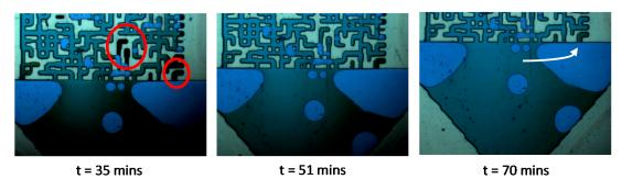
Figure 16. CO<sub>2</sub> invading water-saturated dead-end pores through the oil, in Case 2.
