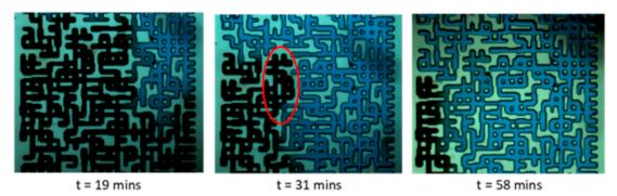
**Figure 9.** CO<sub>2</sub> transport inside the micromodel at a location 4–11 mm from the top of the micromodel, in Case 1.
